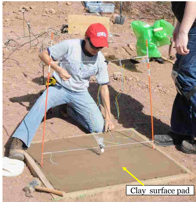
Figure 4.4. Clay surface pad constructed to capture airblast-induced craters
