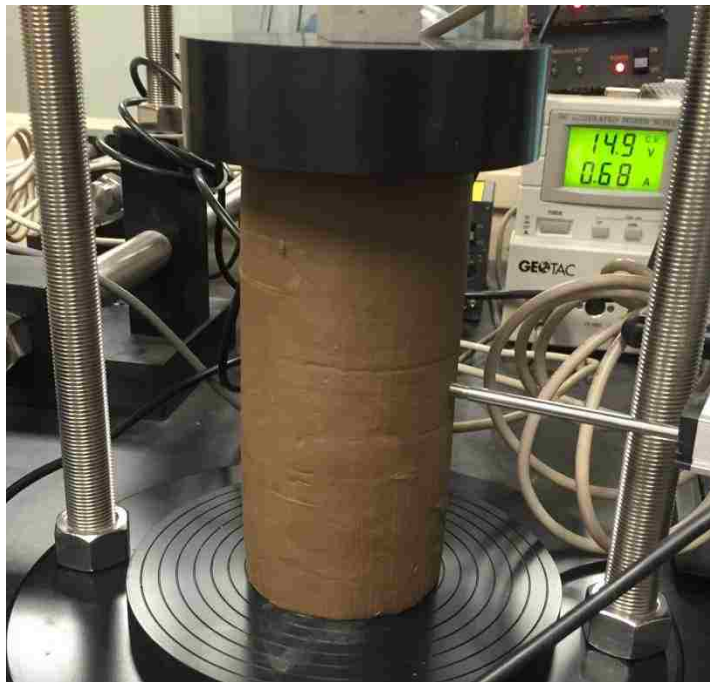
Figure 3.4. Unconfined compressive strength (UCS) testing
